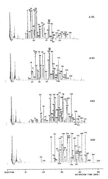
Fig. 2. Temperature programmed capillary ECD chromatograms of Clophen A30, A40, A50 and A60. Component identification by IUPAC numbers and by "u" if yet unknown.
